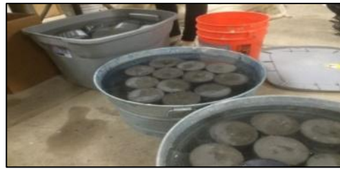
Figure 3: Cylinders under curing process
